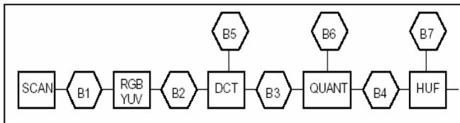
Fig. 2. The block diagram of the JPEG encoder.
