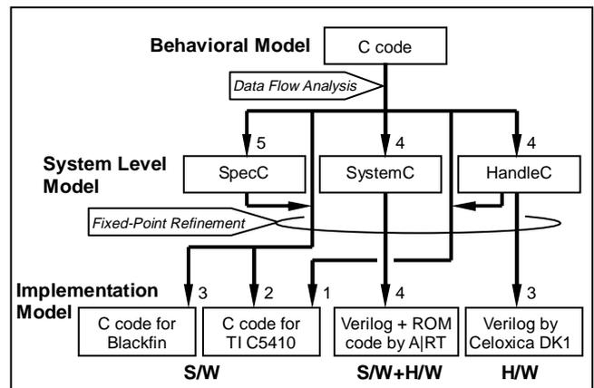
Fig. 1. Design flow for the JPEG encoder. The numbers indicate how many teams were assigned to use the models.
